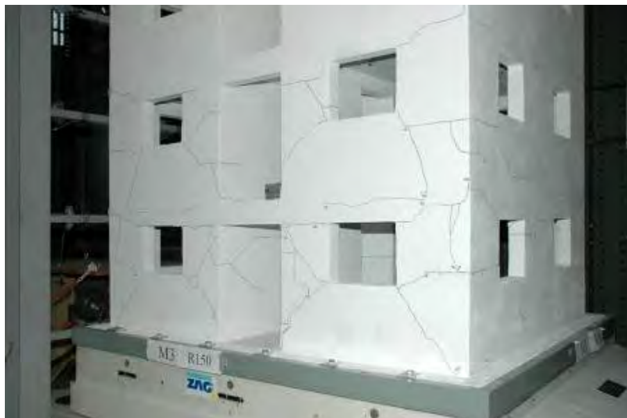
Figure 6.68: Typical diagonally oriented shear cracks in the walls of model M3 at maximum resistance after test run R150 [55].
