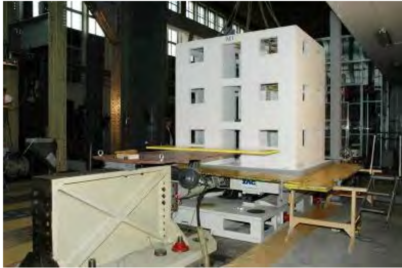
Figure 6.19: Shaking table with one of the models, ready for testing. Steel reaction wall and hydraulic actuator can be seen in front of the table [55].
