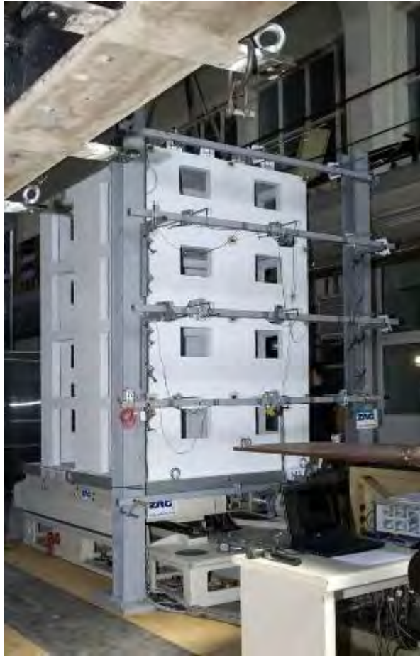
Figure 6.20: Steel supporting frame to fix the displacement transducers during the testing of model M3 [55].
