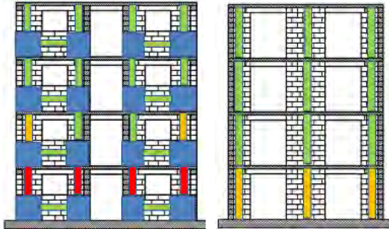
Figure 6.52: Status of link element in step 15 (27,20 mm) with rigid floors. North elevation (on the left) and south elevation (on the right).
