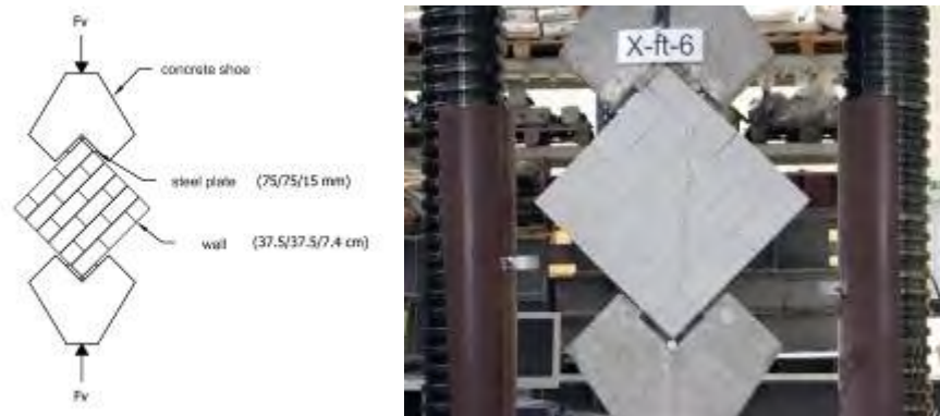
Figure 6.18: Test set-up for the diagonal compression test [55].
